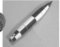
At last glue the nose to the main body of the rocket.
