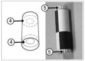
into a tube. Glue the discs 4 inside the top and the bottom of 1. Finally add the connectors 5 to each end of 1.
