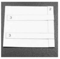
the strips 3 to the backside of part 1. Use the red markers as guidelines. When dry, roll 1
